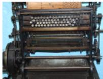
Figure 3: A Jacquard card punch, the tool used to "program" the Jacquard loom [10]
